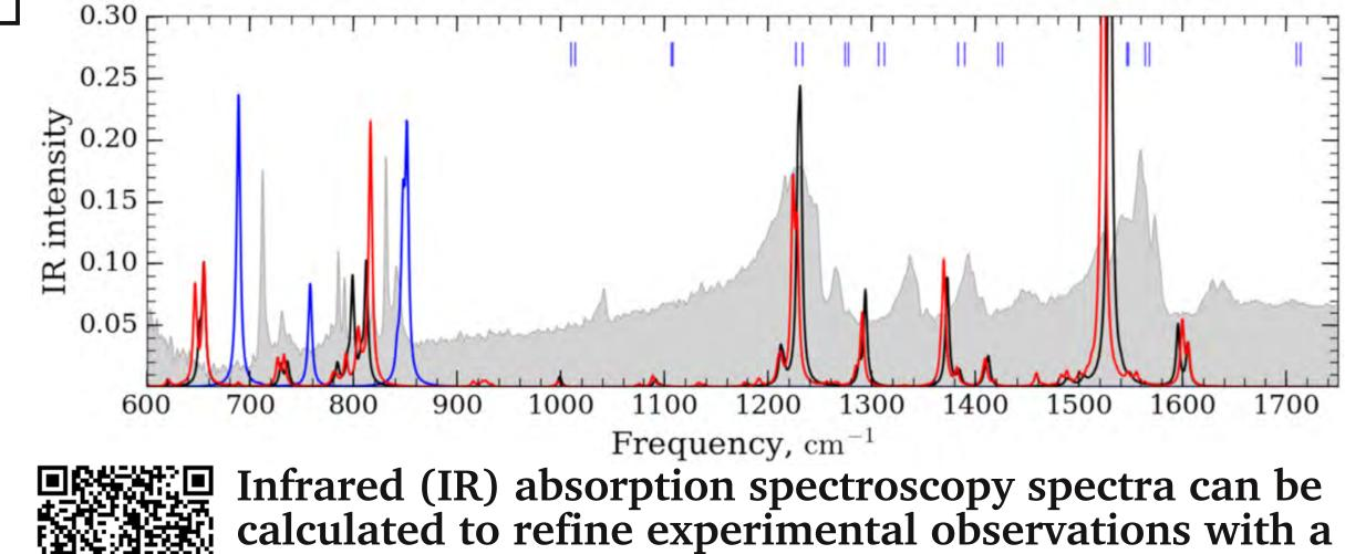
structural model. In this example, mono- and bilayers of PTCDA on Ag(111) are investigated.
