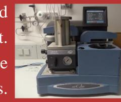
Preliminary investigations are conducted by *in situ* thermal analysis (DSC with pressure chamber,  $T_{max} = 450 \,^{\circ}$ C,  $p_{max} = 70 \,^{\circ}$ bar). *In situ* powder X-ray diffraction gives a deeper insight into the reaction steps and intermediates. Additionally, Raman spectrometry can be operated simultaneously to characterize amorphous components. *In situ* powder neutron diffraction has the advantage to detect light elements like hydrogen during the whole
