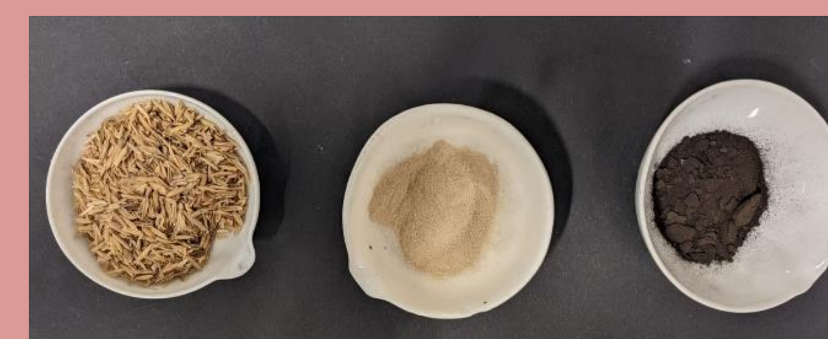
Different processing states starting with rice husks (left), grounded rice husks (mid) and hydrocarbon (right).
